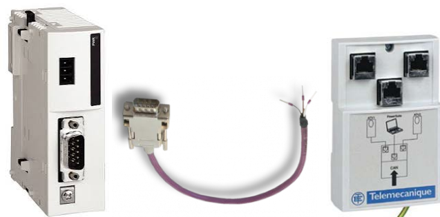
Fig 11. Connection of TWDNC01M and TAP VW3CANTAP.
