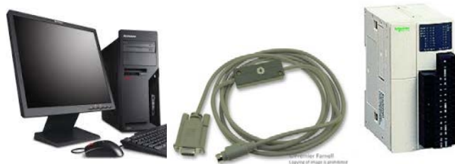
Fig 10. Connection your computer and PLC-TWDLMDA20DRT.
