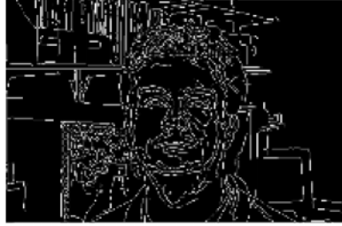
Fig 2. – an edge map obtained by searching for pixels with biggest gradient.
