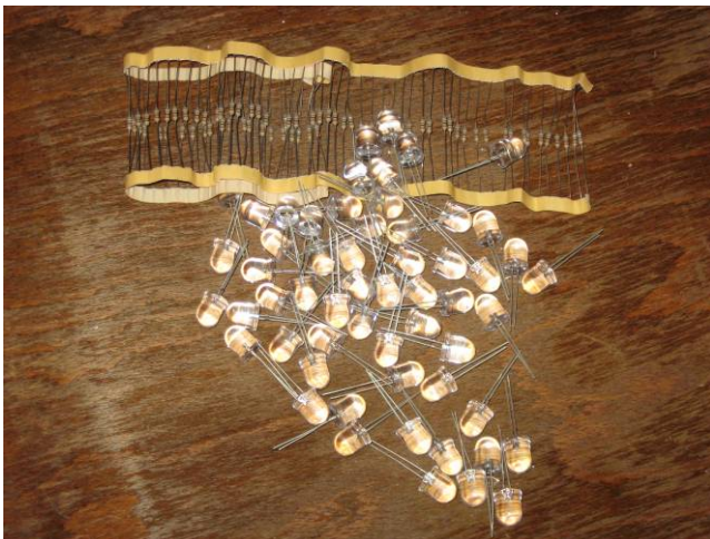
Fig. 3.LED and resistors that are put on the panel
